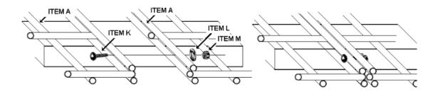
Installation using Garageflex PowerTrack
