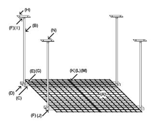
Step 1: If installing through drywall, locate and mark the ceiling joists using either a stud finder or drill
