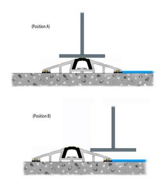
(Position A) The Threshold Seal may be fitted to the floor directly beneath the door so that the door closes on the top of the Threshold Seal.
